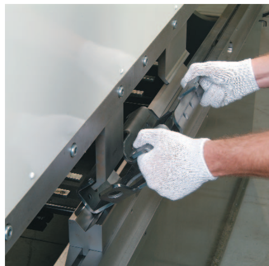
Stage bending of a part with nine bends shows flexibility of even the most basic Pro2.
