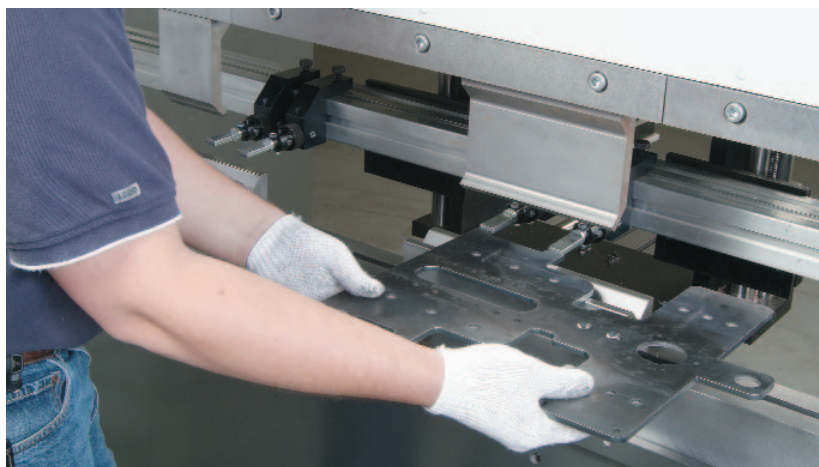
Stage bending of a part with nine bends shows flexibility of even the most basic Pro2.
